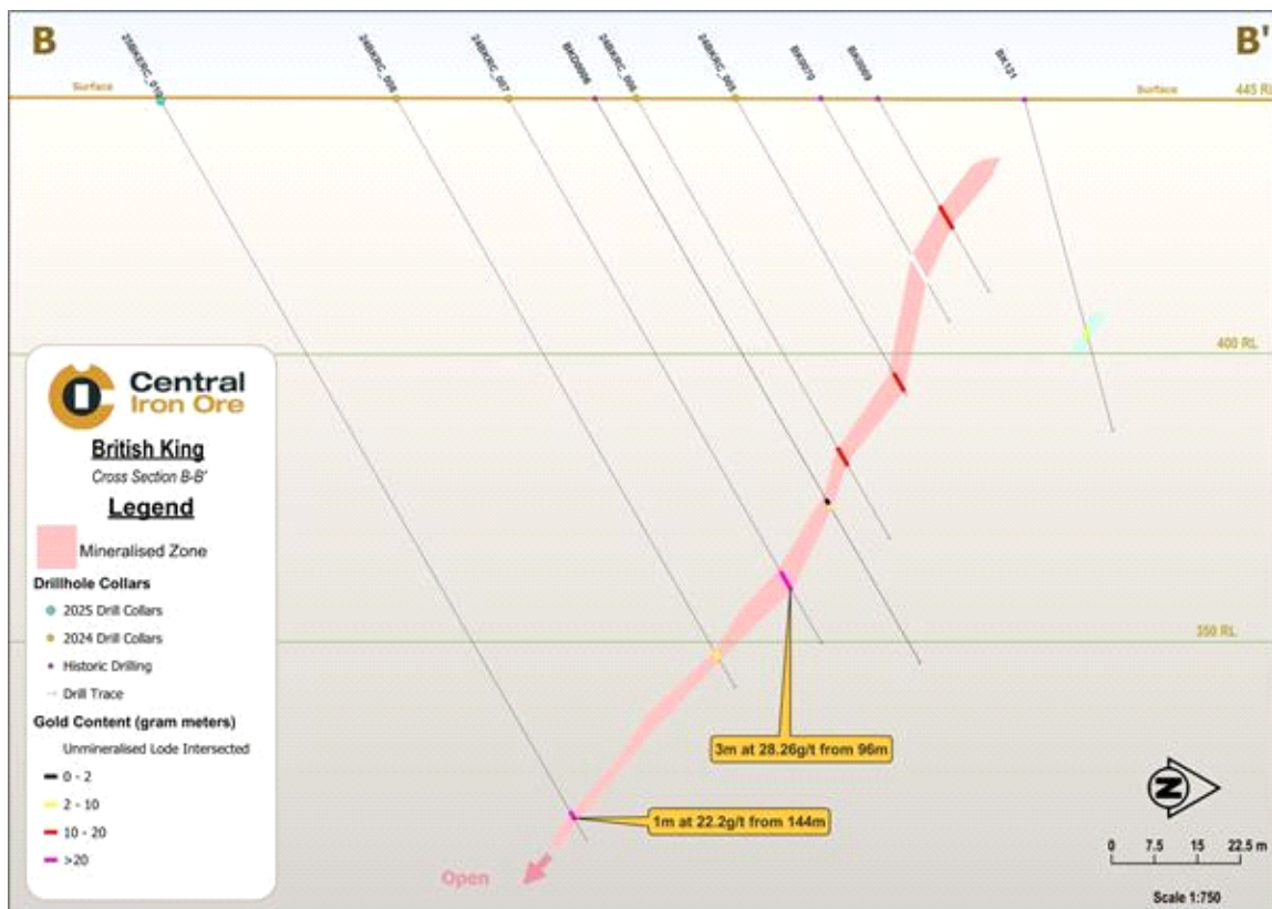
Figure 4. Section B-B': multiple significant high grade intercepts have been identified
